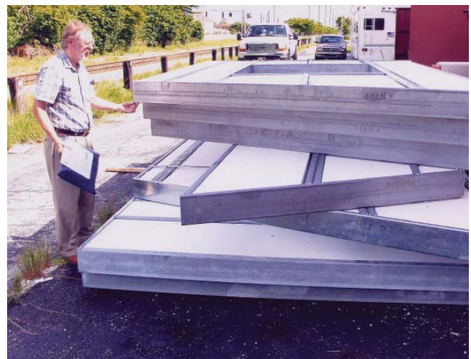
(Fig. 21) The core adds structural strength and rigidity to the overall system.
