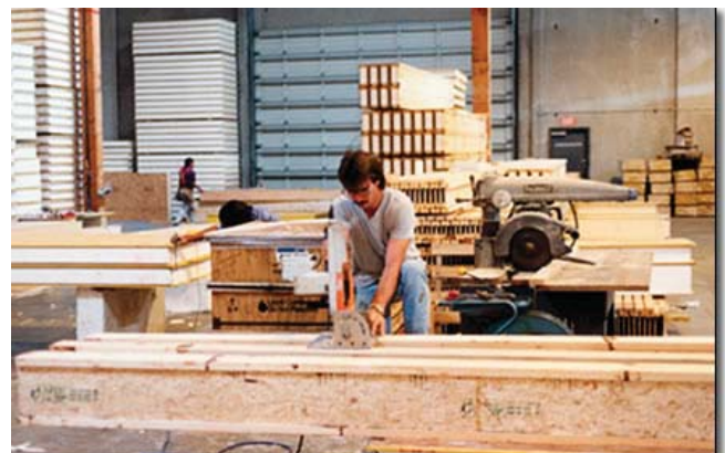
(Fig.9) Structural insulated panel components being made in a factory.
