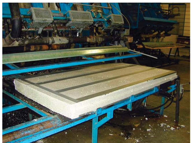
(Figs. 23-24) Steel-framed panels manufactured by Thermasteel, in the factory (bottom) and being laid out on site (top).
