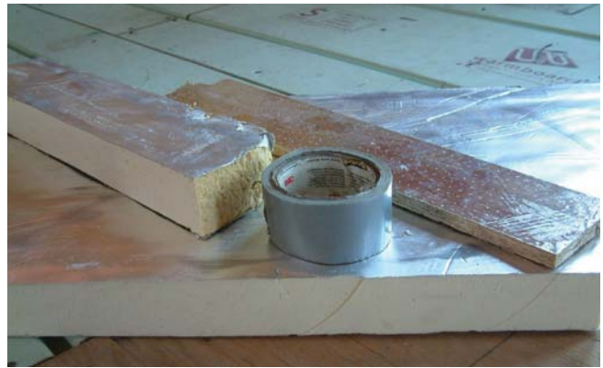
(Fig.5) Radiant barriers come in a variety of forms. The main variable is the backing material.
